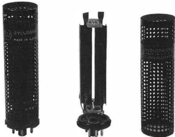
Sylvania 5Z4, RCA 5Z4 elements and perforated cover
