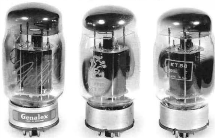
Genalex KT88 (early 1960s with gold script on tube and red decal on base), Genalex KT88 (1970s) and Mullard KT88 (1969 actually a Genalex tube)
