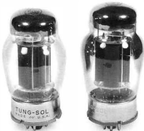
Tung-Sol 6550 (first type 1955 black plate, no holes top getter) and Tung-Sol 6550 (late 1950's black plate, no holes and triple getter)
